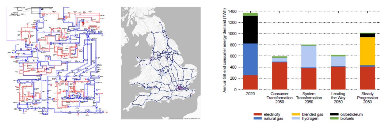
**Network Features**: 572 transmission lines, 758 transformers, 741 nodes (busbars), 270 substations, HVDC link Scottish Boundary
